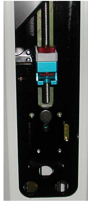
Standard SYRINGE BLOCK for use with sample return
