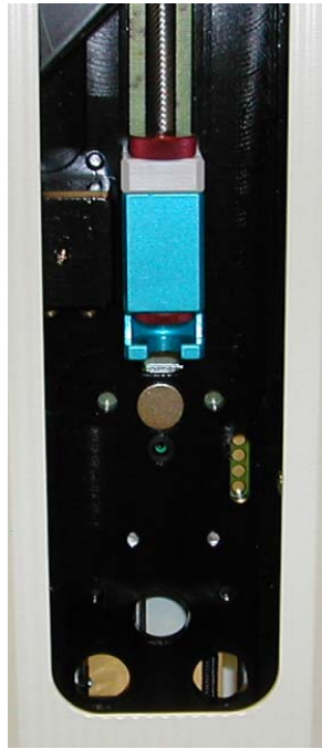
Standard SYRINGE BLOCK for use without sample return
