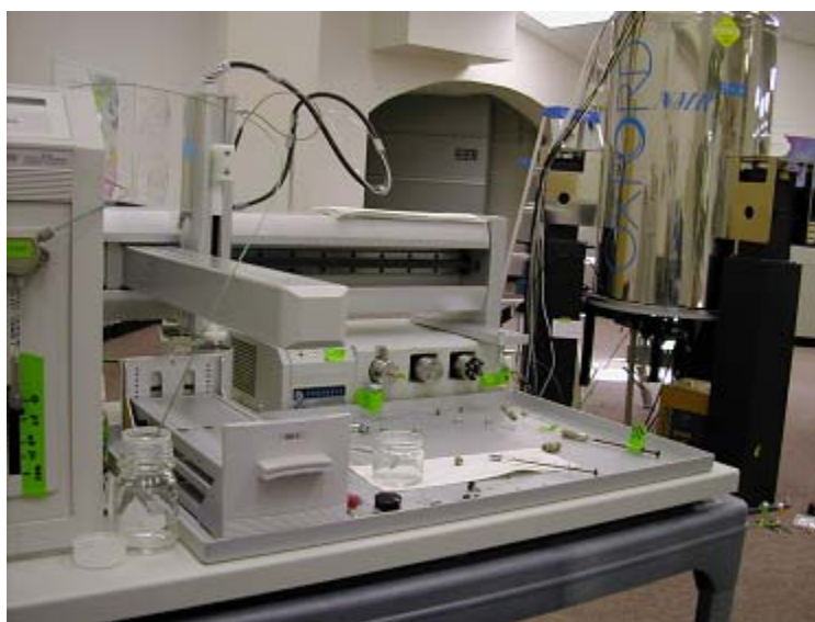
Figure 2. (a) schematic & (b) pictorial illustrations of the Gilson 215/Protasis HTSL platform for \mu VAST/ \mu BEST NMR.
